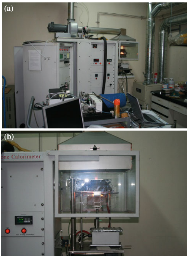
Fig. 1 Experimental set-up of the cone calorimeter. a Cone calorimeter, b cone heater
